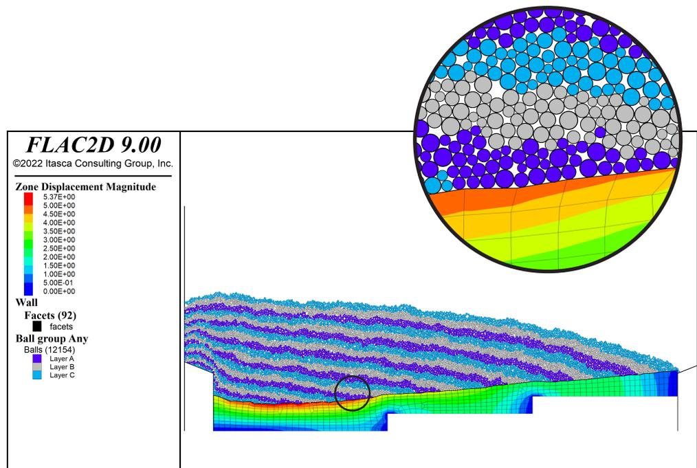
*FLAC2D 9* and *PFC2D 9<sup>4</sup>* can be coupled to leverage the power of both discrete element method (DEM) and continuum modeling. In this project *PFC2D* balls are deposited onto a soft elastic material under large strain conditions.
