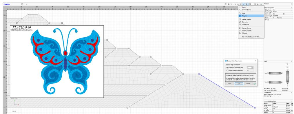
Through sketch sets, *FLAC2D* 9 provides interactive model creation tools for model construction, meshing, and specifying groups. Specify edge and zone size targets and automatically create unstructured or structured meshes. Easily import CAD files, convert them to edges and automatically mesh, as with the butterfly shown in the insert.
